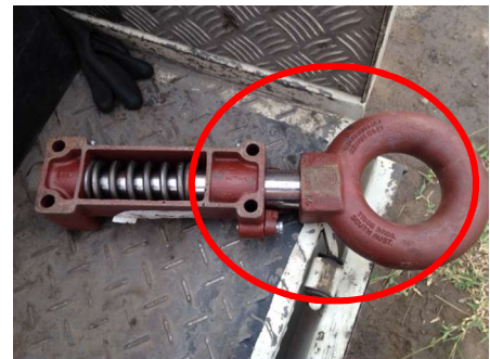
Picture 4 – The above picture shows where a new ring feeder shaft has been slightly bent due to towing abuse.
