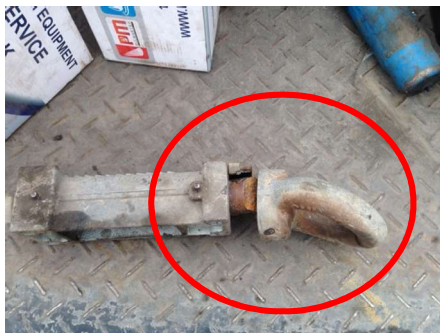
Picture 1 – Clearly shows a ring feeder that has failed due to excessive speed in rough conditions.
