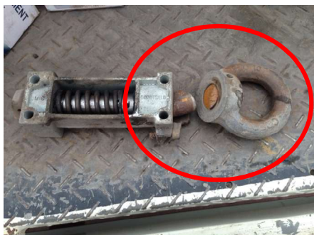
Picture 3 – The above picture again shows where the ring feeder shaft has been bent through jack-knifing the trailer, causing the shaft to fail.
